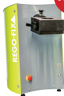
PGS 25 Unit Automatic clamping unit for single sizes
